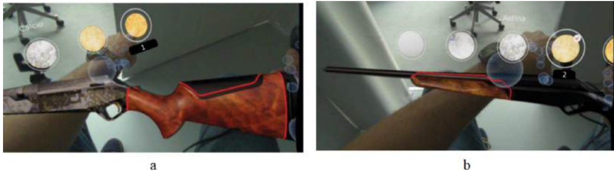
Fig. 8. MR application developed for a sporting rifle. The application presents several rifle stock (a) and forend (b) materials. For these components, only real wood and GAN wood are selectable through numbers on the screen.
