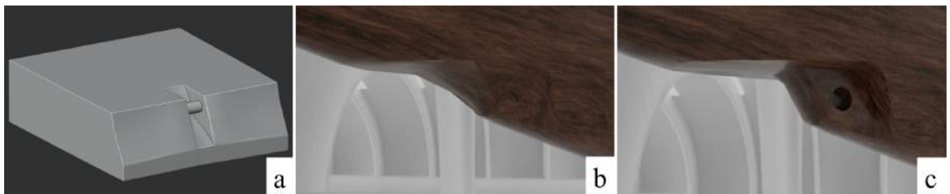
Fig. 3. Elements relative to the employment of the Boolean modifier. Figure (a) shows the 3D-modelled cutting tool used for the sling hole on the rifle stock. Without this cutter, the Shrinkwrap modifier produces artefacts (b). Figure (c) shows the Shrinkwrap modifier action corrected thanks to the cutting tool showed in (a).
