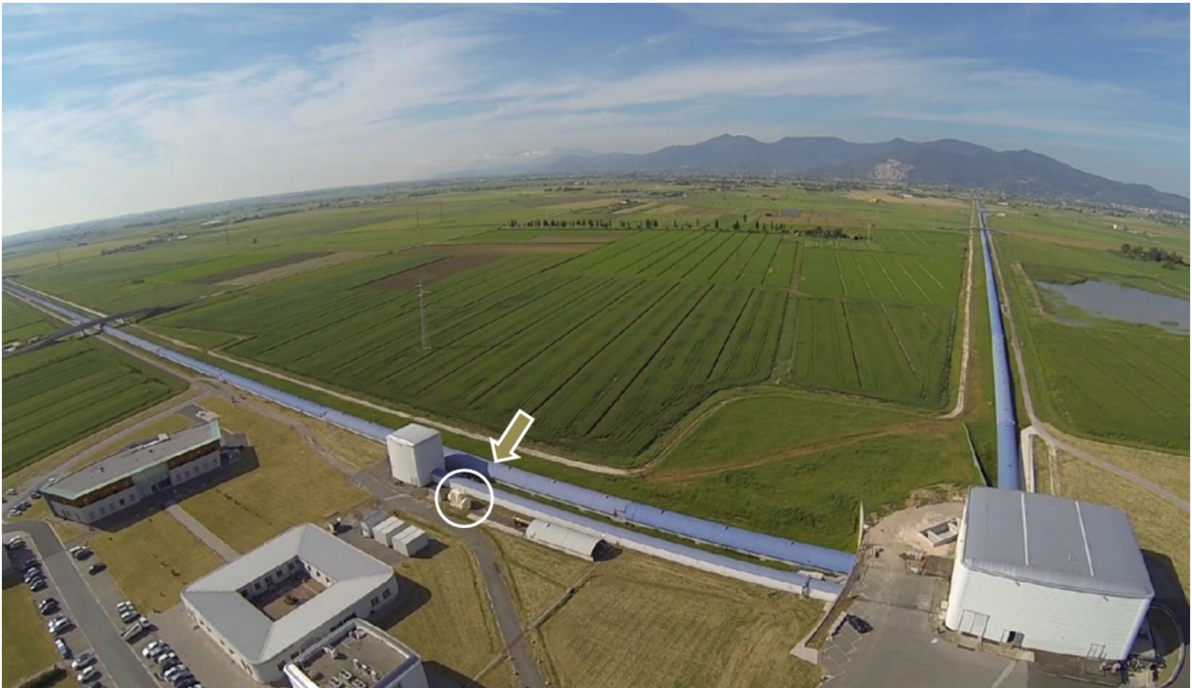
Fig. 2 The picture shows Virgo (Pisa), with its 3 km-long orthogonal arms. Besides Virgo and indicated by an arrow and a circle, lays the 3 m long cryogenic bar Explorer, which
