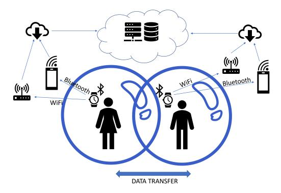
**Figure 1.** The BubbleBox system is composed of a device, i.e., a wristband to log unsafe contacts, an app, to pair devices and the identities of people wearing them, and a server infrastructure to store data and make it available of the authorized medical personnel.
