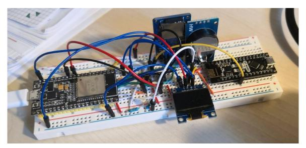
**Figure 4.** A breadboard with the device components, used to simulate the wristband and, thus, test the distance estimation performed by such device.
