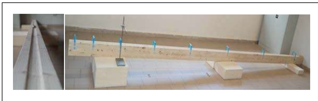
Fig. 3. The inclined plane with the bells and the pendulum built and used at the Liceo Scientifico "F. Sbordone" in Naples. Source: own experiments images.
