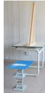
Fig. 5 The experimental apparatus for the reconstruction of the parabolic trajectory of the bullet. Source: own experiments images
