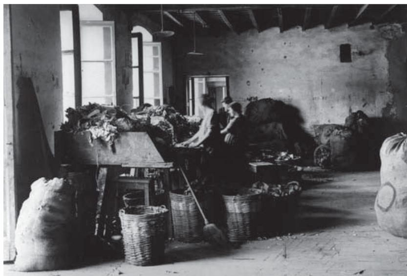
Fig. 1. Selection of rags , ca. 2 nd half of 19 th century (Pigna Paper Mill Historical Archive).
