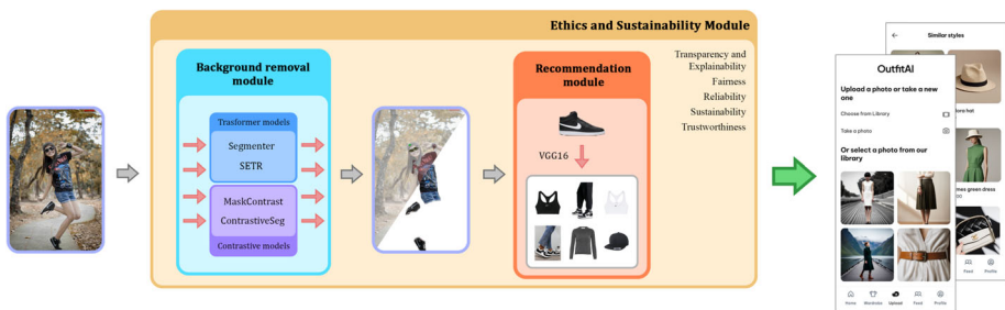
Fig. 1 OutfitAI System Architecture. This diagram illustrates the comprehensive architecture of OutfitAI, showing its three core modules. The Background Removal Module uses transformer-based neural networks to accurately segment fashion items from complex backgrounds, ensuring high quality input for feature extraction. The Recommender Module uses similarity algorithms to match these processed images with a wide range of products from partner e-tailers, providing users with personalised fashion recommendations. Finally, the Ethics and Sustainability Module is guided by the ethical guidelines for trustworthy AI, embedding sustainable practices and ethical considerations into every aspect of the system, from data handling to product promotion
